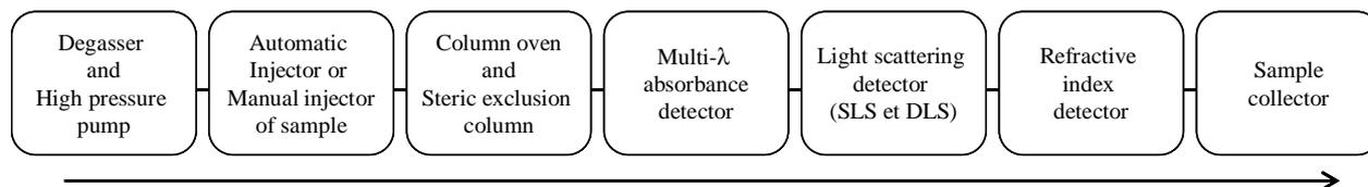
The **degasser** “**SHIMADZU DGU 20A**” enables to degas the -previously filtered at 0.1µm- column solvents.
