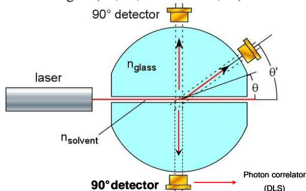
According to the Rayleigh-Debye-Gans model, the intensity *I* of the light scattered by the solution is directly proportional to the total concentration *c* (g/ml) and to the average molar mass *M<sub>w</sub>* (g/mol) of the macromolecules in the solution:
